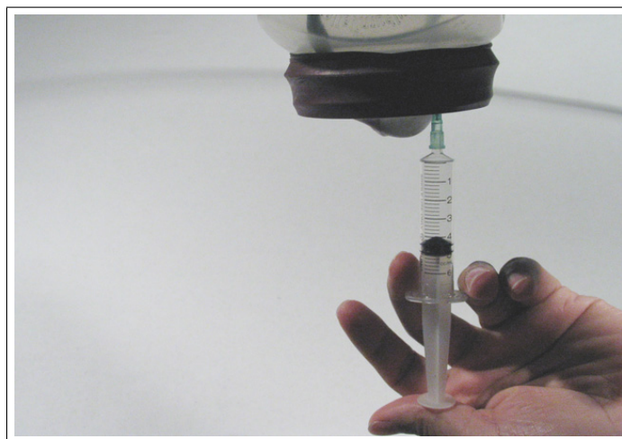
Figure B.8: The syringe is emptied into the container upside down due to hydrogen's relative density
