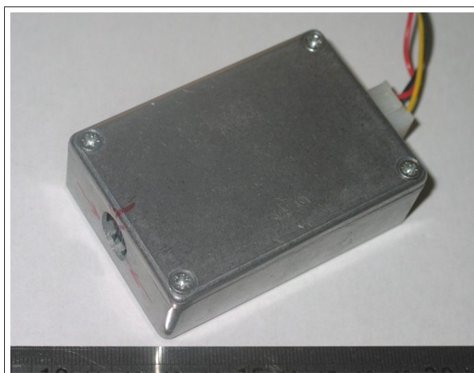
Figure 4.12: Panterra-CAT in an aluminium enclosure, the sensing hole is located on the side
